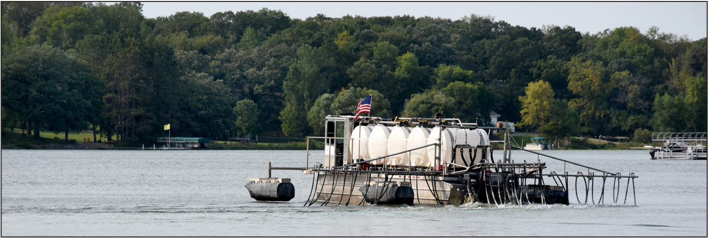
Guided by GPS, a SOLitude Lake Management crew applied alum to targeted areas of Blue Lake. A Clean Water Fund grant from the Minnesota Board of Water and Soil Resources supported the Isanti SWCD project, which addresses in-lake phosphorus. The 2022 treatment wrapped up on Sept. 15. The Blue Lake Improvement District provided the 25% grant match.
