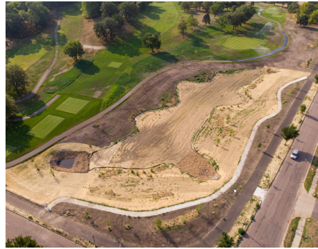
Previously untreated runoff from 612 acres now flows from east to west through Columbia Golf Course and Columbia Park, where it is diverted to a treatment pond, a dry basin, and then an infiltration basin before it re-enters the stormwater sewer system and continues on for 1.2 miles to the Mississippi River. The Clean Water Fund-supported project is slated to wrap up this month. Photo Credits: Mississippi WMO
