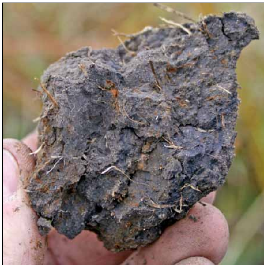
Figure 25. Redox features can be small and difficult to see within a dark soil layer.
