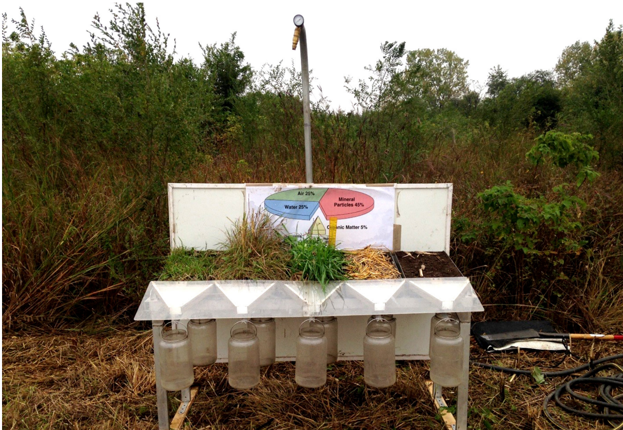
A rainfall simulator compares cropping systems, tillage systems, runoff and infiltration. It was purchased in 2017 with funds from the Renville County Economic Development Authority and local capacity grants from Renville, Redwood and McLeod soil and water conservation districts.
