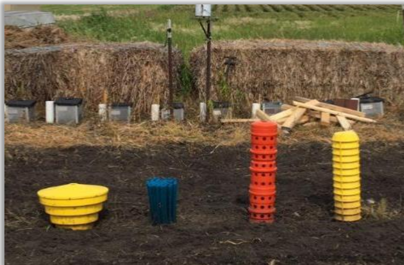
Surface inlets evaluated in this study. From left to right: (1) Ag-Solutions® QuickDrain® low profile inlet (QD), (2) AgriDrain® wick inlet (AD), (3) Hickenbottom® standard inlet (HB), and (4) Ag-Solutions® standard inlet (AS).
